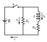
A coil with an inductance of 2.0 H and a resistance of  $10~\Omega$  is suddenly connected to an ideal battery with  $\epsilon = 100~V$ . At t = 0.10~s after the connection is made, what is the rate at which (a) energy is being stored in the magnetic field, (b) thermal energy is appearing in the resistance, and (c) energy is being delivered by the battery?
